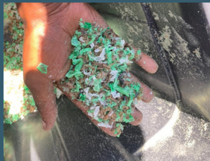
4a. Mixed, damaged, contaminated, and non-recyclable plastics are shredded and mixed with non-recyclable glass to make driveway pavers, construction blocks, and more
