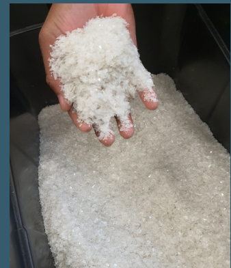
4b. Clean, "good" plastics are cleaned, rolled, and granulated and re-sold back into the supply chain by grade and color
