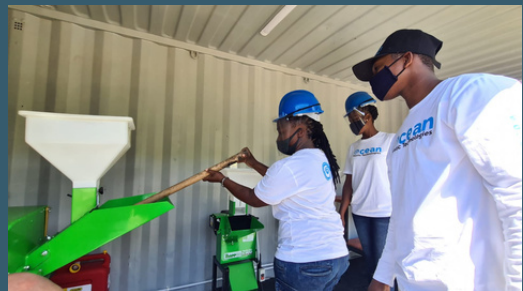
3. Plastic is sorted by quality, then plastic type, then color, then it is cleaned and processed either partially or fully at the MRP
