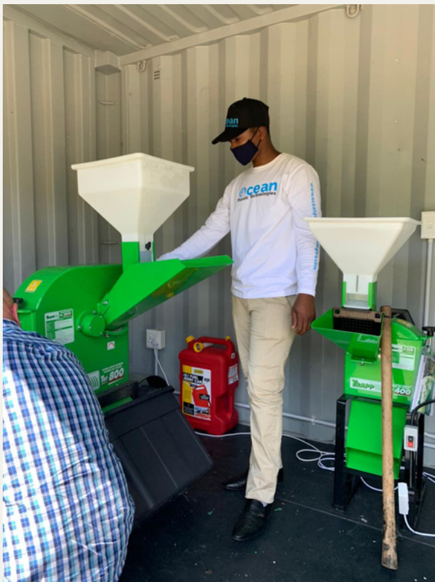
Recycling of ocean plastic at an Ocean Plastic Technologies Micro Recycling Plant (MRP)
